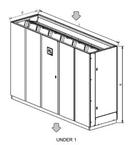
Necessary clearance on right-hand side (in front of the cabinet): 900 mm min.
